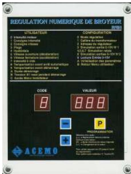
There are two set data for respectively user and configuration in controller. Normally the controller is in the user-menu, as the configuration is blocked by a code.
